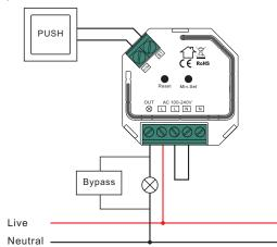
**NOTE:** Switch connected to the S1 terminal activates the basic functionality of the dimmer (turning the light on/off, dimming).
